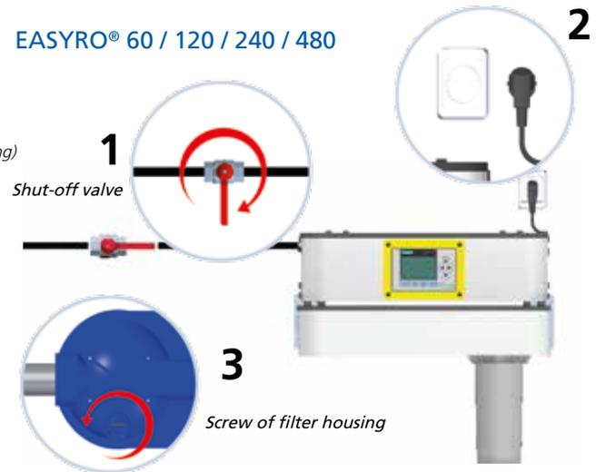
Close the main water shut-off valve (1) and disconnect the power plug (2) of the EASYRO® from the mains power supply.
